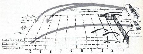
Triple spading: 1A and 2A strips of surface soil are removed, and later moved to cover the last two strips at 9A and 10A; 1B strip of subsoil is removed, and added finally to 10B; 1C strip of substratum is spaded; 2B subsoil is spaded, mixed, and placed above 1C; 3A surface soil is put above moved subsoil in place of the original 1A.
